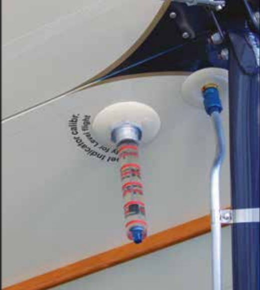
A float ball in a viewing tube indicates fuel level. Also note the filigree paint work.
