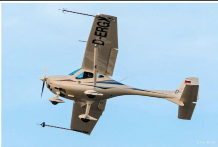
Figure 4: messWERK Remos GX with Flight test instrumentation (Foto: Uwe Bethke)
