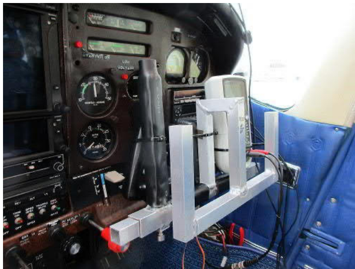
Figure 3: Secondary yoke with strain gages for force measurements (Foto: author)
