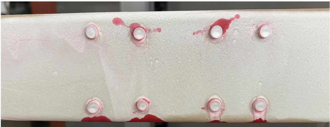
FIGURE 4: EXAMPLE 2 - CRACK LOCATIONS - FWD SIDE OF SPAR
